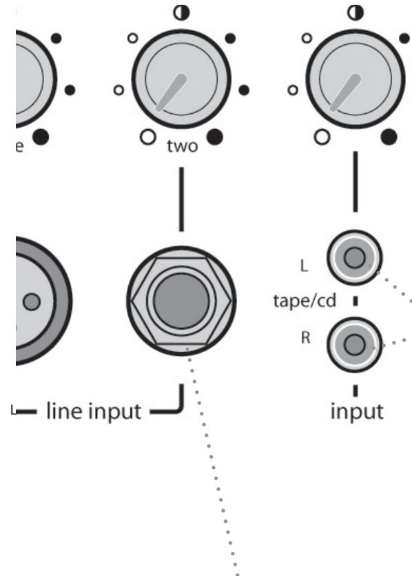
Plug any line-level source with a 1/4" phone plug (tape player, music instrument, etc) into line input two. The knob above the jack controls the volume level.
