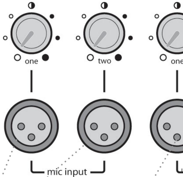
Plug a microphone with an XLR connector into mic input one or two. The knob above the jack controls the volume level.
