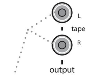
Connect RCA outputs to a tape player's input to record the sound system.
