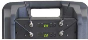
**▲ Note:** Remove antennas before transporting to avoid damage.
