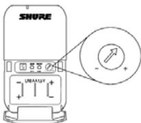
Rotate the audio gain adjustment to increase (+) or decrease (-) the gain until desired level is reached.
