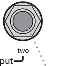
Connect line output two to a tape player's input to record the sound system.
