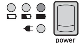
**Battery Power** (upper LED's): The green light indicates the battery is at or near full charge and ready to use. The yellow light means 20-30% usage remains, and red means less than 15% remains and that the battery should be charged before use (see "Charging the battery").
