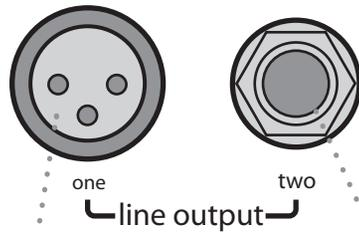
Connect line output one to the balanced input of another system for daisy-chain applications.
