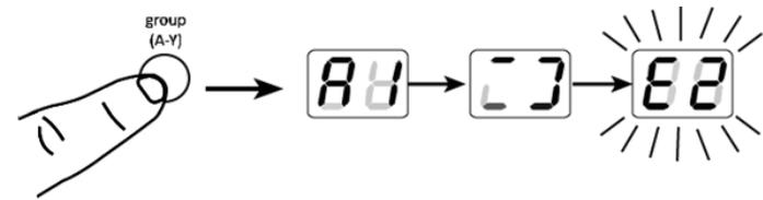
2. **Transmitter Setup:** Transmitter group and channel must be manually set to match the receiver.
